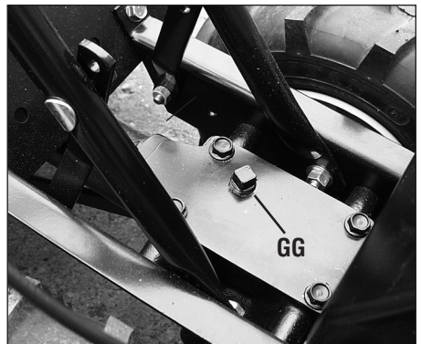
Fig. 2-11: Remove gear oil fill plug.
